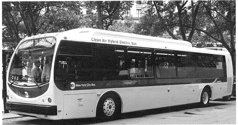
The New York Metro Transit Authority has ordered 90 HEV buses that feature C30 microturbines. The C30s generate electricity to charge batteries on the HEV buses.
