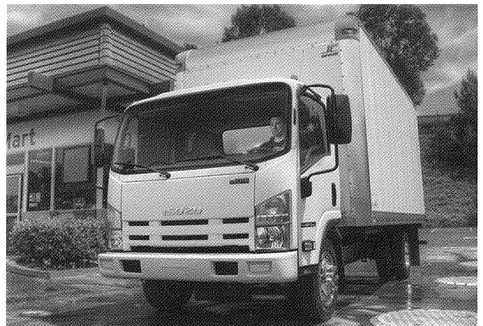
Wrightspeed’s The Route REV truck features a Capstone C30 microturbine, which serves as the range-extending power source once the battery is depleted.
